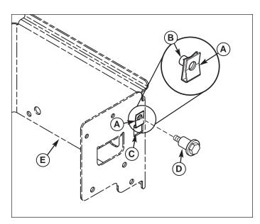
Figure 1. Install Spacer (left side shown)
